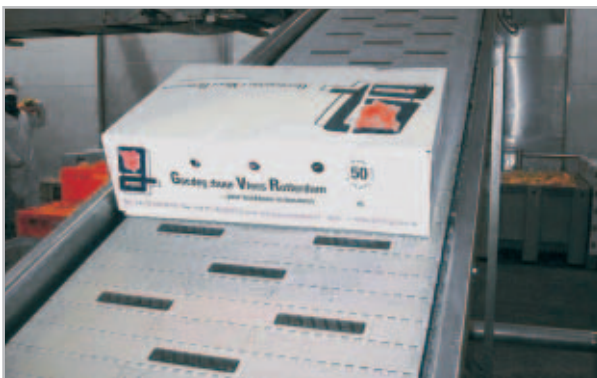
Safe 25° decline for slippery heavy packages in a meat plant.
