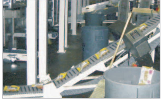
Snack food bag very gently conveyed, no tearing of bags as with previous flighted belt.
