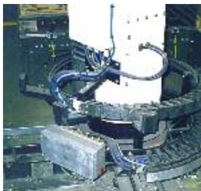
Spiral and rotary movement TwisterChain®
