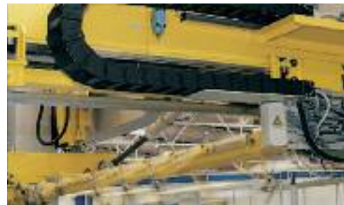
System E4 partially unsupported - please consult igus regarding this type of configuration.
