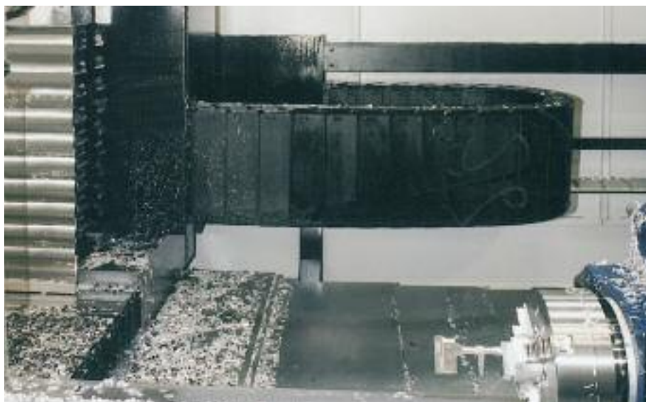
System E4 Energy Tube in direct chip area E4/light
