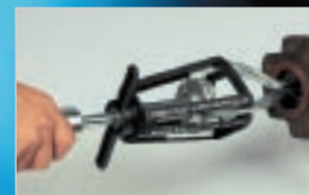
Pilot bearing removal from crankshaft (Model PM16)
