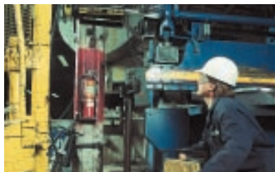
A 50-ton hydraulic puller easily removes the main drive gear from this metal forming brake press.
