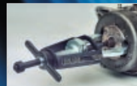
Clutch removal (Model 204)
