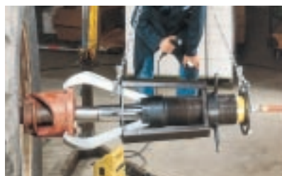
Hub removal from shaft. (Model PHES-116)
