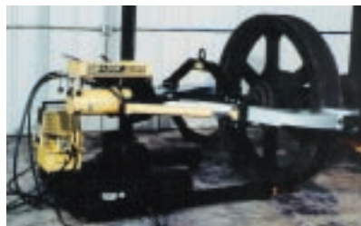
A 100 ton puller hydraulic puller quickly and easily removes this drive sheave from its shaft.
