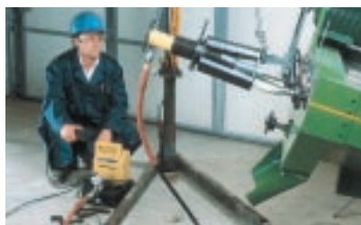
Sprocket removal from shaft. (Model PHES-110)
